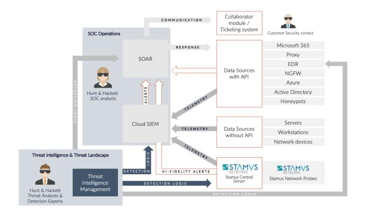
For Hunt & Hackett's flexible service deployment model, the Stamus Security Platform built-in VPN was an important capability. This enables remote network probes to be securely connected to the central server, supporting a variety of deployment architectures.
