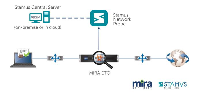
In a "network inline - appliance passive" configuration, the ETO sits in the middle of the traffic flow – between the client and the server. When the SSL/TLS handshake occurs, the ETO actively participates in the handshake to insert itself in the TLS flow, it then decrypts the flow and passes the plaintext data over to the Stamus Network Probe for analysis. Then it reencrypts the data and sends it on to the destination, maintaining the end-to-end connection in an encrypted form.
